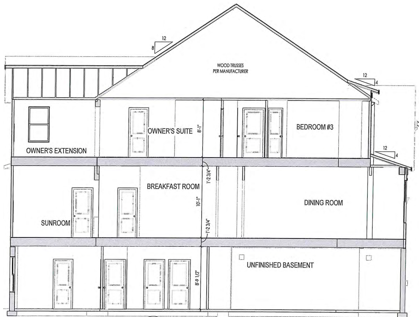
A BUILDING SECTION THRU FOYER 5.01 1/8" = 1'-0"
