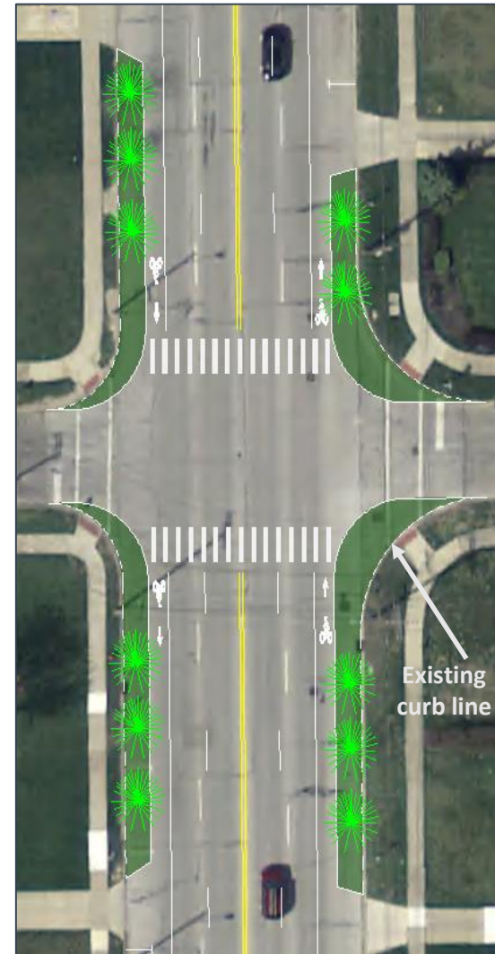
Figure 14: Bump outs and crosswalks at Hillbrook Road intersection
